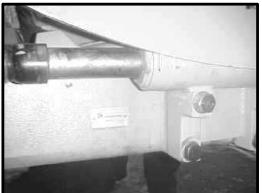
The front axle serial number is stamped on a plate mounted on the axle.
