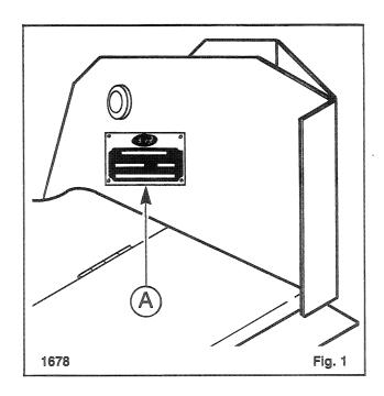
A vehicle identification plate is located on the inside of the fuel tank above the engine compartment cover at the rear of the machine (fig. 1 item A).
