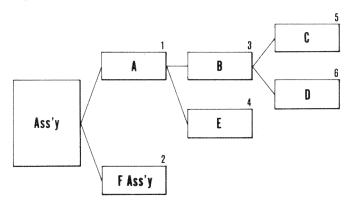
In the network, the sequence of the procedural steps are given in arabic numbers on the right top of each block. For example, when it is necessary to remove part [] from the assembly, the steps for removal should be [] [] [] [] [] This is an assembly of witch the disassembling procedure is described separately. For assembly, the sequence is presented in the same manner, under each section, as for disassembly.
