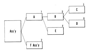
In the network, the sequence of the procedural steps are given in arabic numbers on the right top of each block. For example, when it is necessary to remove part D from the assembly, the steps for removal should be  $A \Rightarrow B \Rightarrow D$ . Or, to remove part E the step is  $A \Rightarrow E$ . F Ass'y This is an assembly of which the disassembling procedure is described separately. For assembly, the sequence is presented in the same manner, under each section, as for disassembly.
