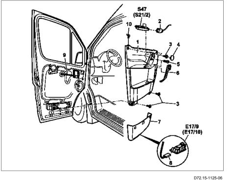
E17/9 Driver entrance/exit lamp (with code (LB9) Illuminated exit) Passenger entrance/exit lamp (with code (LB9) E17/10 Illuminated exit)
