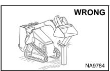
Never work on loader with lift arms up unless lift arms are held by an approved lift arm support. Replace if damaged.
