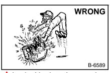
Lead-acid batteries produce flammable and explosive gases.
