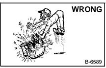
Lead-acid batteries produce flammable and explosive gases.
