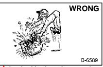
Lead-acid batteries produce flammable and explosive gases.
