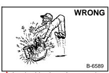
Lead-acid batteries produce flammable and explosive gases.
