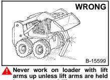
arms up unless lift arms are held by an approved lift arm support device. Replace if damaged. Never modify equipment or add attachments not approved by Bobcat Company.
