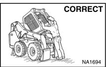
Lise the correct procedure to lift or lower operator cab.
