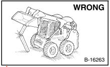
Never work on I oader with lift arms up unless lift arms are held by an approved lift arm support device. Replace if damaged.
