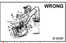
Lead-acid batteries produce flammable and explosive gases.
