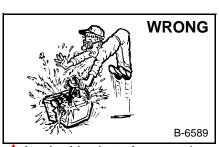
Lead-acid batteries produce flammable and explosive gases.
