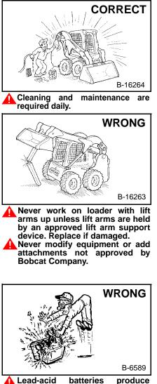
Lead-acid batteries produce flammable and explosive gases. Keep arcs, sparks, flames and lighted tobacco away from batteries.
