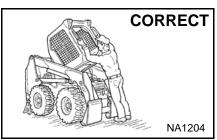
Lightharpoonup Use the correct procedure to lift or lower operator cab.
