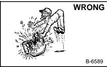
Lead-acid batteries produce flammable and explosive gases.
