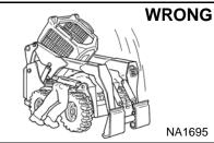
Disconnecting or loosening any hydraulic tubeline, hose, fitting, component or a part failure can cause lift arms to drop. Do not go under lift arms when raised unless supported by an approved lift arm support. Replace it if damaged.
