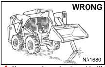
Never work on loader with lift arms up unless lift arms are held by an approved lift arm support. Replace if damaged. Never modify equipment or add
