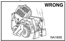
Disconnecting or loosening any hydraulic tubeline, hose, fitting, component or a part failure can cause lift arms to drop. Do not go under lift arms when raised unless supported by an approved lift arm support. Replace it if damaged.
