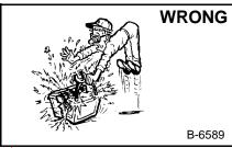
Lead-acid batteries produce flammable and explosive gases.
