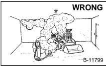
Have good ventilation when welding or grinding painted parts.
