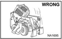
Disconnecting or loosening any hydraulic tubeline, hose, fitting, component or a part failure can cause lift arms to drop. Do not go under lift arms when raised unless supported by an approved lift arm support device. Replace it if damaged.
