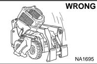
Disconnecting or loosening any hydraulic tubeline, hose, fitting, component or a part failure can cause lift arms to drop. Do not go under lift arms when raised unless supported by an approved lift arm support device. Replace it if damaged.
