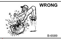
Lead-acid batteries produce flammable and explosive gases.
