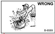
Lead-acid batteries produce flammable and explosive gases.
