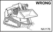
Never work on loader with lift arms up unless lift arms are held by an approved lift arm support. Replace if damaged.
