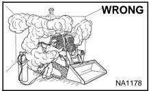
A Have good ventilation when welding or grinding painted parts.
