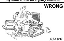
A Stop, cool and clean engine of flammable materials before checking fluids.
