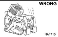
Disconnecting or loosening any hydraulic tubeline, hose, fitting, component or a part failure can cause lift arms to drop. Do not go under lift arms when raised unless supported by an approved lift arm support. Replace it if damaged.
