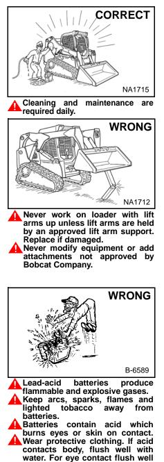
Maintenance procedures which are given in the Operation & Maintenance Manual can be performed by the owner/ operator without any specific technical training. Maintenance procedures which are **not** in the Operation & Maintenance Manual must be performed **ONLY BY QUALIFIED BOBCAT SERVICE PERSONNEL.** Always use genuine Bobcat replacement parts. The Service Safety Training Course is available from your Bobcat dealer.
