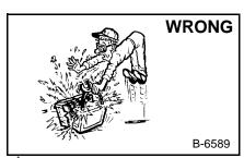
Lead-acid batteries produce flammable and explosive gases.
