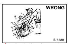
Lead-acid batteries produce flammable and explosive gases.
