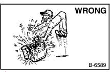
produce batteries Lead-acid flammable and explosive gases.
