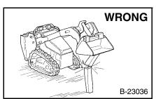
Never work on I oader with lift arms up unless lift arms are held by an approved lift arm support dévice. Replace if damaged.
