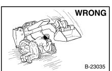
Disconnecting or loosening any hydraulic tubeline, hose, fitting, component or a part failure can cause lift arms to drop. Do not go under lift arms when raised supported by a approved lift arm support device. Replace it if damaged.
