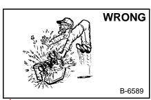
Lead-acid batteries produce flammable and explosive gases.
