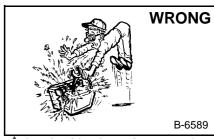
Lead-acid batteries produce flammable and explosive gases.
