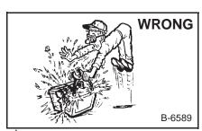
Lead-acid batteries produce flammable and explosive gases.
