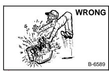
Lead-acid batteries produce flammable and explosive gases.
