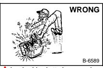
Lead-acid batteries produce flammable and explosive gases.
