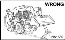
Never work on loader with lift of arms up unless lift arms are held Z by an approved lift arm support device. Replace if damaged.
