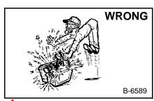
Lead-acid batteries produce flammable and explosive gases.
