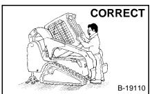
Use the correct procedure to lift to lower operator cab.
