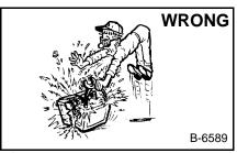
Lead-acid batteries produce flammable and explosive gases.
