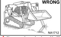
Never work on loader with lift arms up unless lift arms are held by an approved lift arm support. Replace if damaged. Never modify equipment or add
