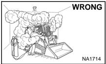
Alave good ventilation when welding or grinding painted parts.
