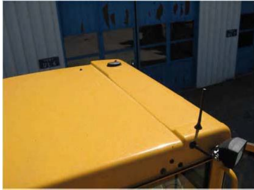
Fig. 2 Antennas mounted on the rear cab roof. GPS/GSM to the left side, satelite to the right side in the picture
