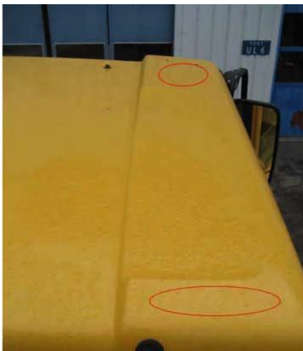
Fig. 1 Suggested antenna positions on roof.
