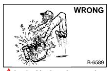
Lead-acid batteries produce flammable and explosive gases.
