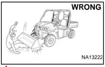
Disconnecting or loosening any hydraulic tubeline, hose, fitting, component or a part failure can cause attachment arm to drop.
