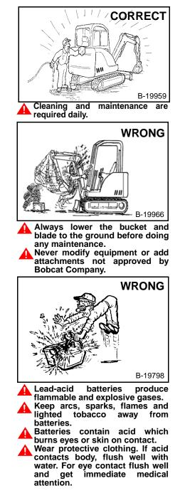
Maintenance procedures which are given in the Operation & Maintenance Manual can be performed by the owner/ operator without any specific technical training. Maintenance procedures which are **not** in the Operation & Maintenance Manual must be performed **ONLY BY QUALIFIED BOBCAT SERVICE PERSONNEL. Always use genuine Bobcat replacement parts.** The Service Safety Training Course is available from your Bobcat dealer.
