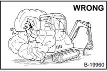
Vent exhaust to outside when engine must be run for service. Exhaust system must be tightly sealed. Exhaust fumes can kill without warning.
