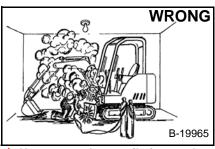
Have good ventilation when welding or grinding painted parts. Wear dust mask when grinding painted parts. Toxic dust and gas can be produced.
