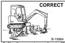
Use the correct procedure to lift and support the excavator.
