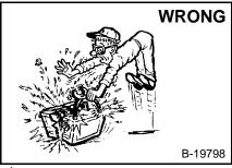
Lead-acid batteries produce flammable and explosive gases.
