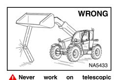
handler with boom up unless boom is held by an approved boom stop. Replace if damaged. Never modify equipment or add attachments not approved by **Bobcat Company.**
