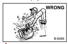
produce Lead-acid batteries flammable and explosive gases. Keep arcs, sparks, flames and
